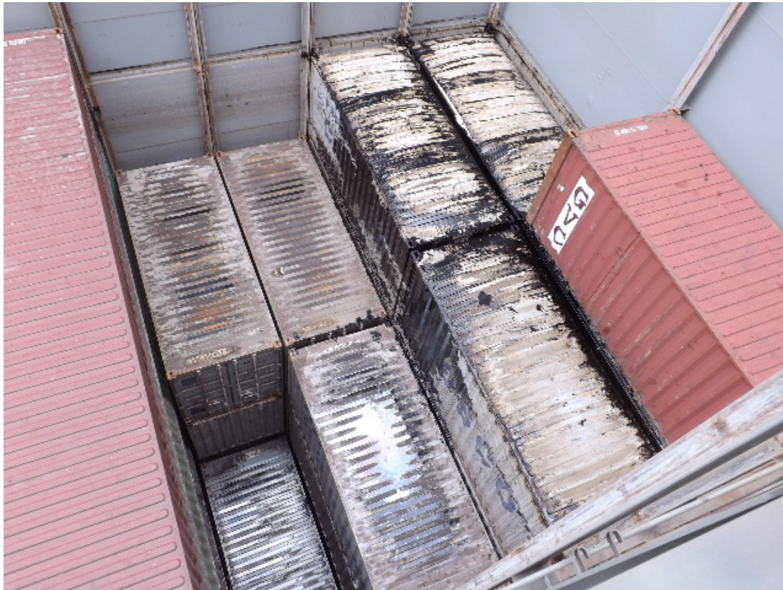
View of wet, contaminated, overweight and bulging containers in hold n.4
